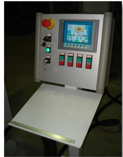
Simple PLC control with touch-panel, status and error messages, clear control panel
